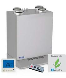
Air handling unit in heat- and sound-insulated casing with electric heater and kitchen hood. Air capacity up to  $270 \, m^3/h$ , heat recovery efficiency up to 95%.
